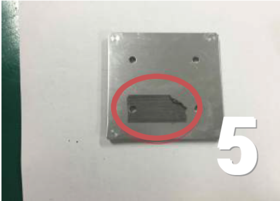
Remove residual tape on the back-plate.
