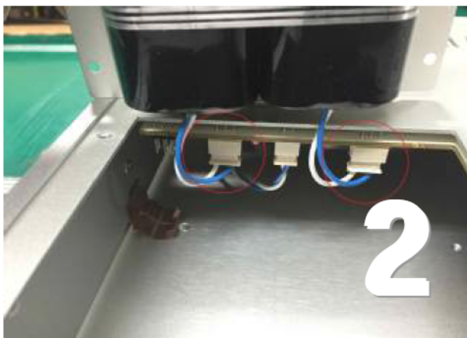
Remove the outer two connectors by pulling down. Leave the center connector alone.
