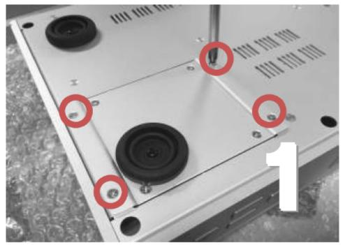
Remove the outer four Phillips screws carefully
