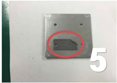
Remove residual tape on the back-plate.
